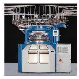
The knitting head is incorporated onto Orizio's new standard frame fitted with an integrated "Millennium" control panel which visibly shows the following information:
